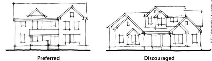
Figure 13: Roof and Eave Lines
