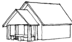
Gable roof - front gable porch
